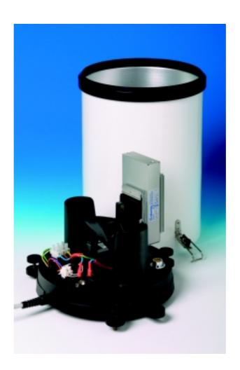
This instrument uses a tipping-bucket mechanism to produce a contact closure every time it receives a predetermined small quantity of rainfall (0.2 mm).
